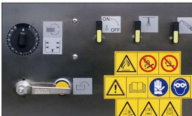
Position the dirty-clean lever in the rinse position (horizontal) for clean solvent and press the rinse button for the desired time for this operation. This way the dispenser nozzles of the washing spray jet system will spray clean solvent into the tub and the blower nozzles will deliver air.
