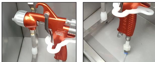
2. Raise the lid of the tub. Press the trigger of the spray gun and use the nylon clip to block the trigger of the spray gun.
