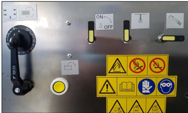
Set the washing timer by turning it clockwise to the desired time. The solvent aspirated from the recirculation solvent tank will begin to come out of the dispenser nozzles and the spray gun nozzle of the spray jet nozzle system inside the tub to perform further washing of the parts, while the blower nozzles will deliver air.
