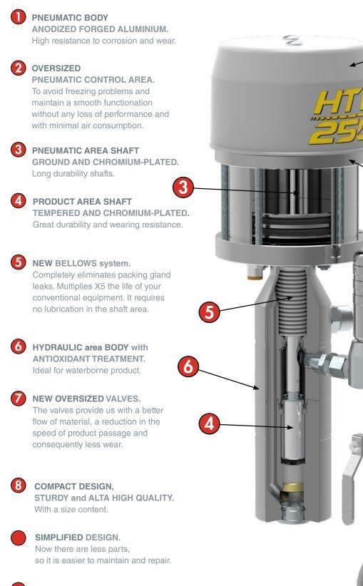
Pump and Atomization regulation SYSTEM HIGH PRECISION.
